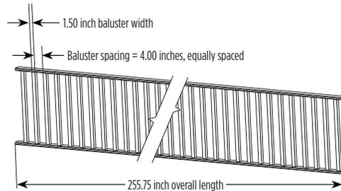
Calculate the number of balusters needed for a handrail measuring 255.75 inches long. The space between balusters is to be about 4 inches. Each baluster is 1-1/2 inches wide.
