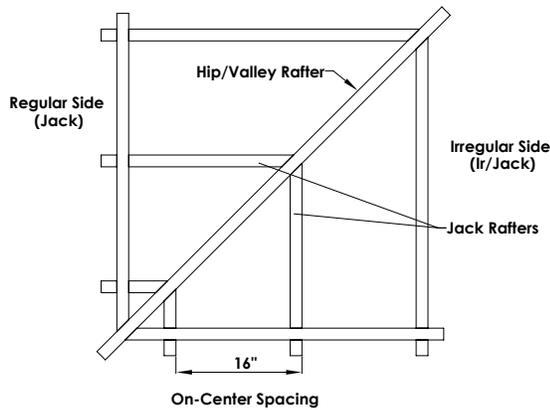
Calculate the lengths of the common, hip/valley and jack rafters (jack rafters at 16 inch on-center). The roof's pitch is 11/12 and half the total span is 7 feet.
